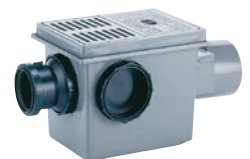
110/3 with three-sided connection option, DN 70 inflow
